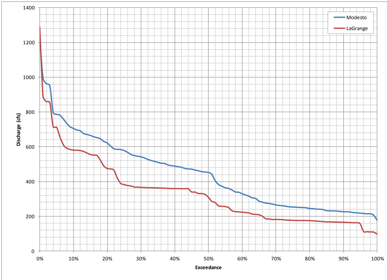
Figure 10. October flow duration curve for the USGS Gages at La Grange and Modesto for the period 2003-2012.
