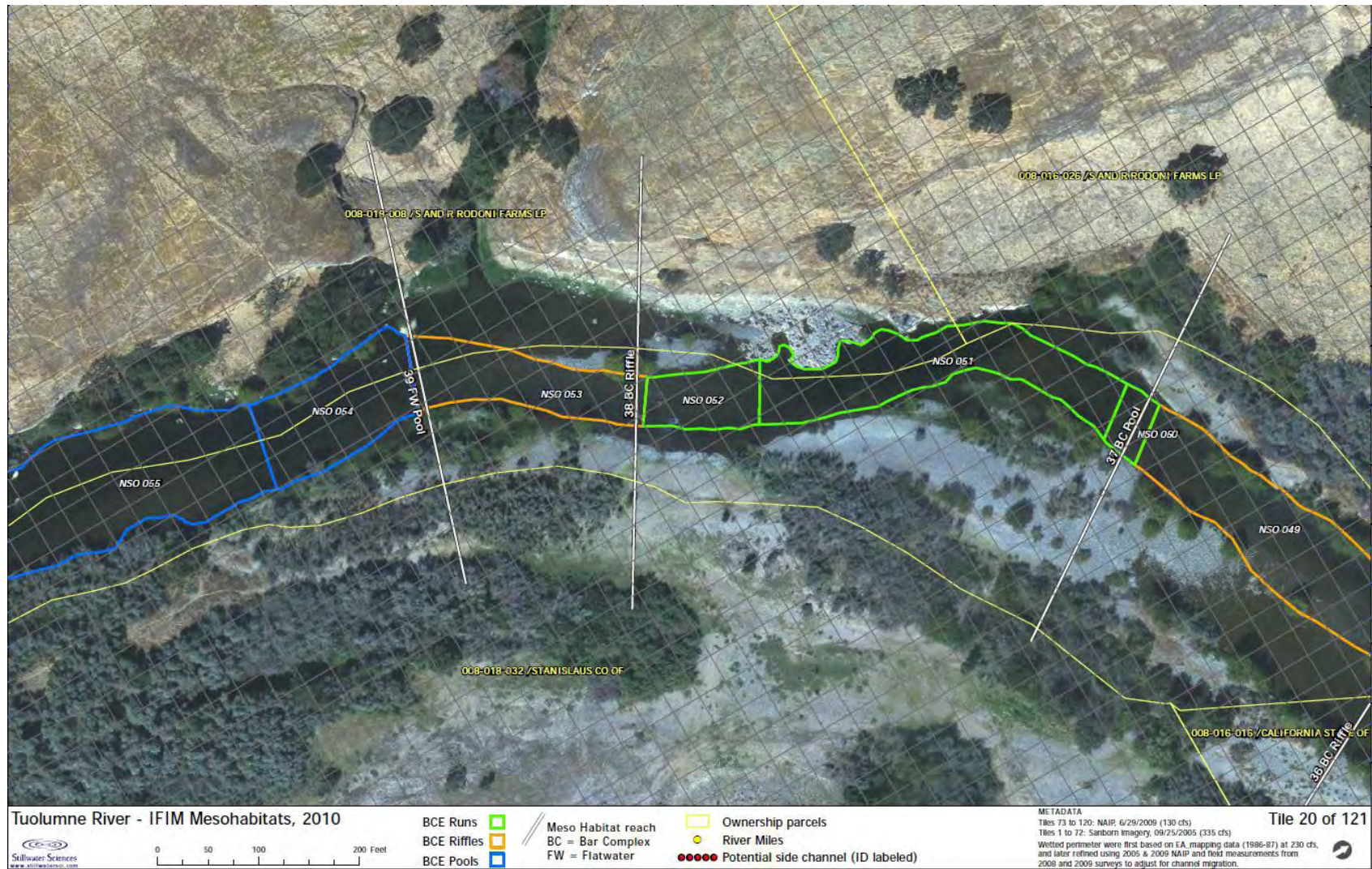
Figure 3. Example aerial photo showing grid used during random sampling site selection, and subdivision of pool into head, body, and tail.
