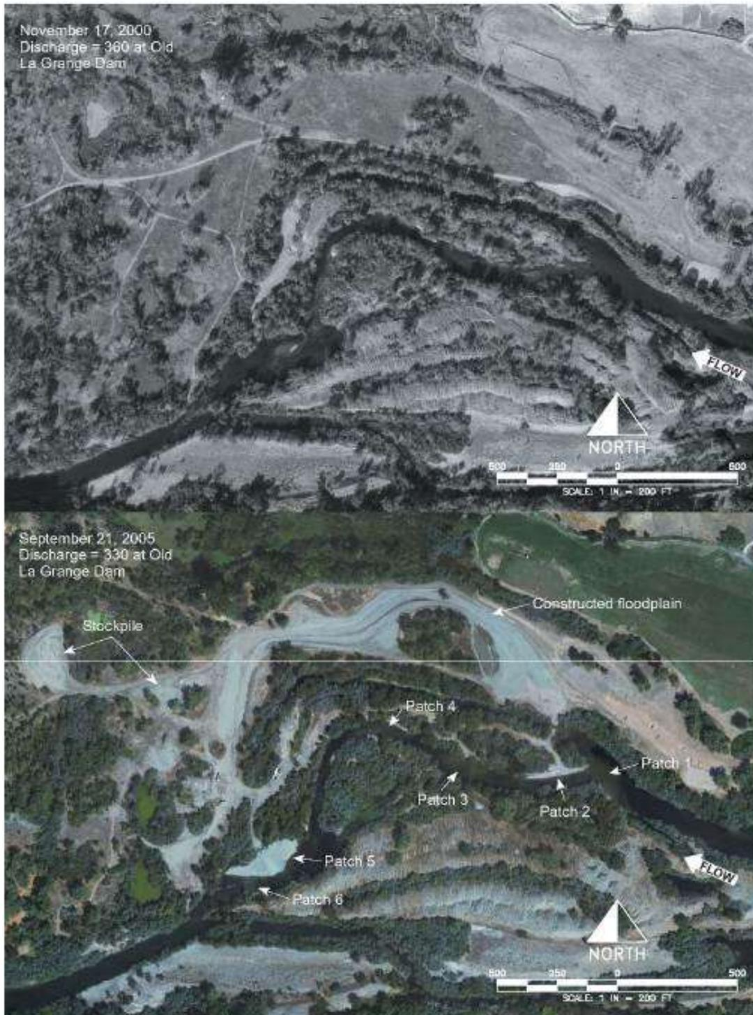
Figure 6. Pre- (November 17, 2000) and post- (September 21, 2005) construction aerial photographs for Bobcat Flat RM 43 Phase I project area.
