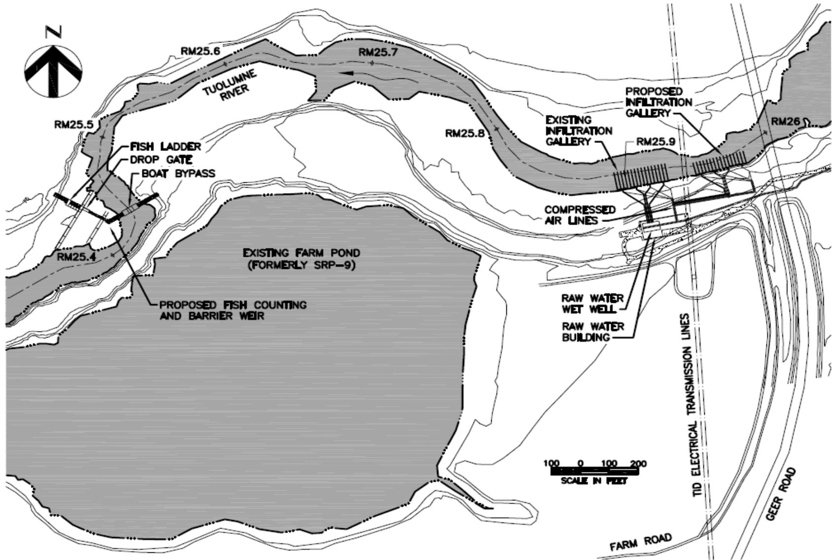
Figure 3.1-1. Location of proposed take-out/put-in (boat bypass) facility.
