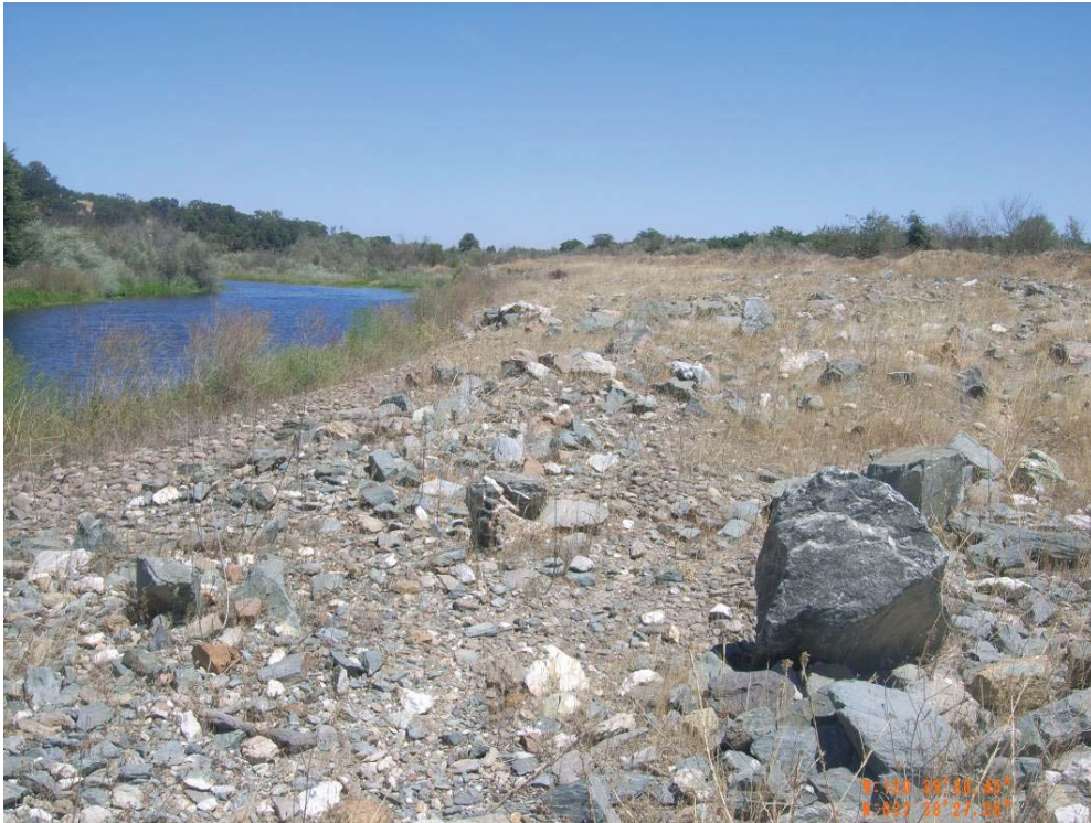
Figure 7. Mannings n is equal to .05.
