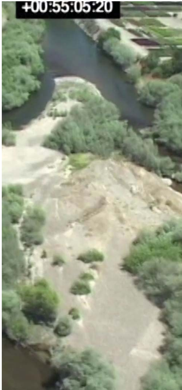
Figure 4. Mannings n is equal to .04.
