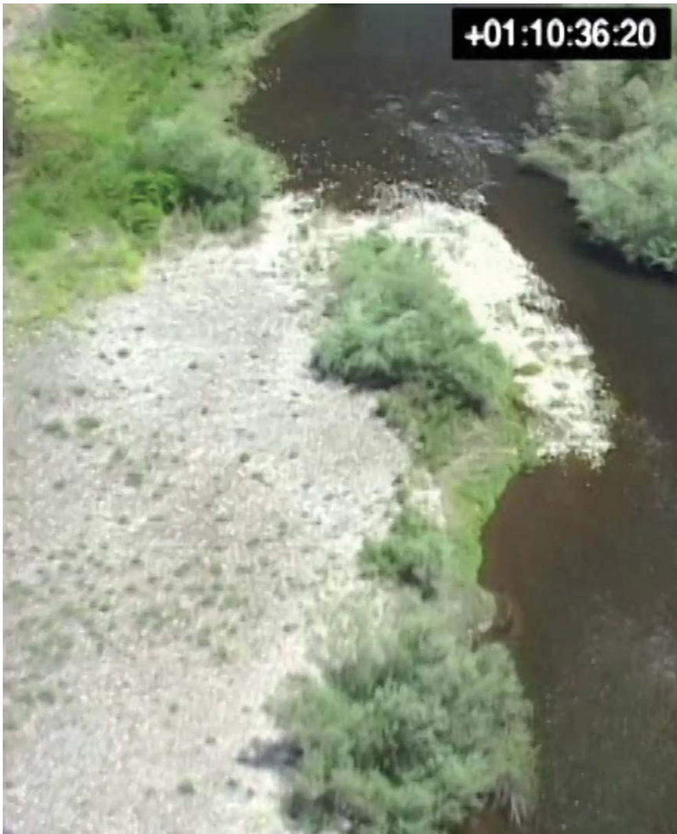
Figure 9. Mannings n is equal to .05.
