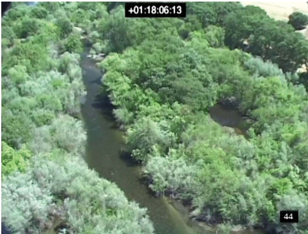
Figure 24. Mannings n is equal to .10.
