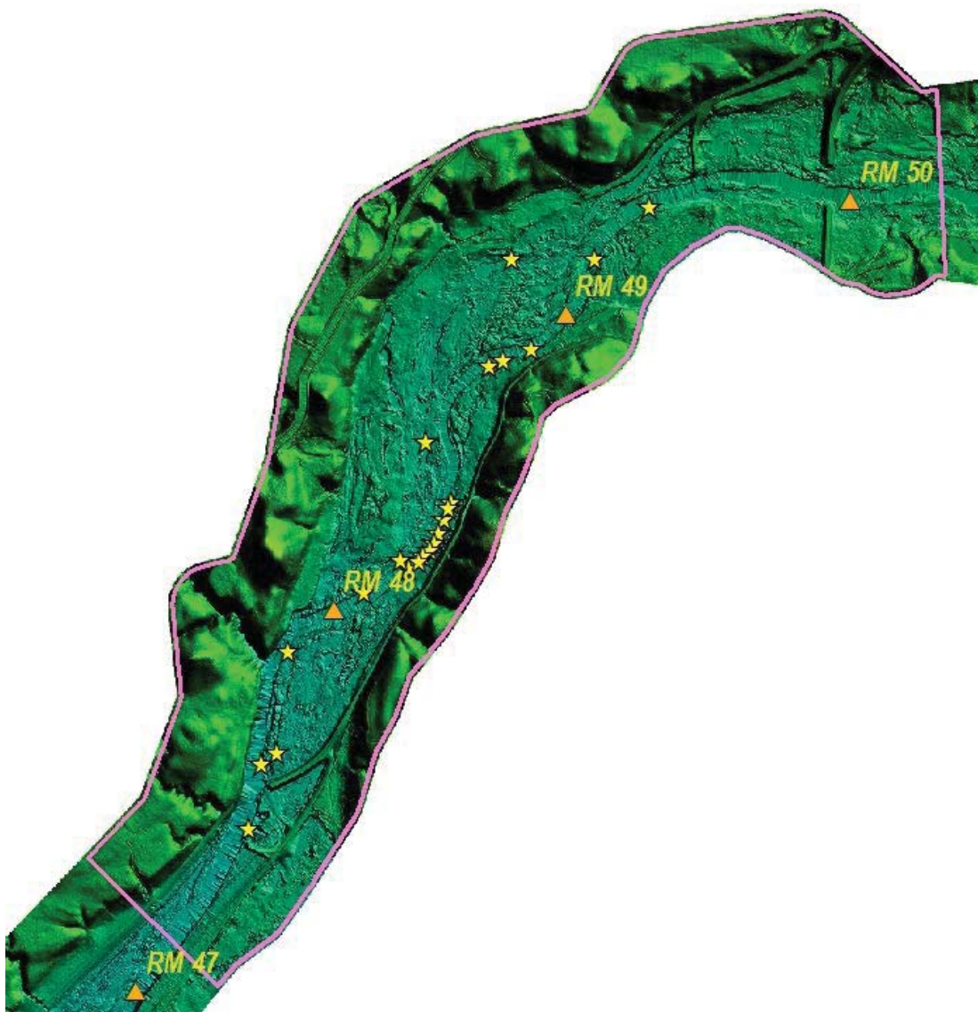
Figure 1. The extent of the TUFLOW model used for cell size sensitivity analysis. Yellow stars represent the locations of water level measurements recorded at a steady flow of 3,000 cfs for the Pulse Flow Study (Stillwater Sciences 2012).
