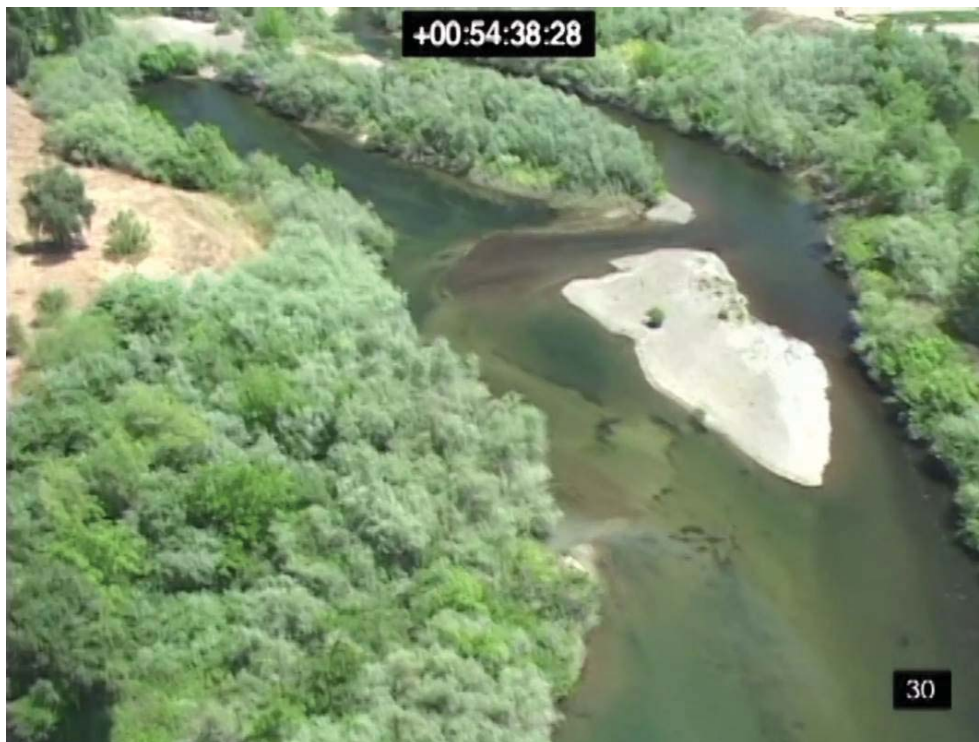
Figure 23. Mannings n is equal to .10.
