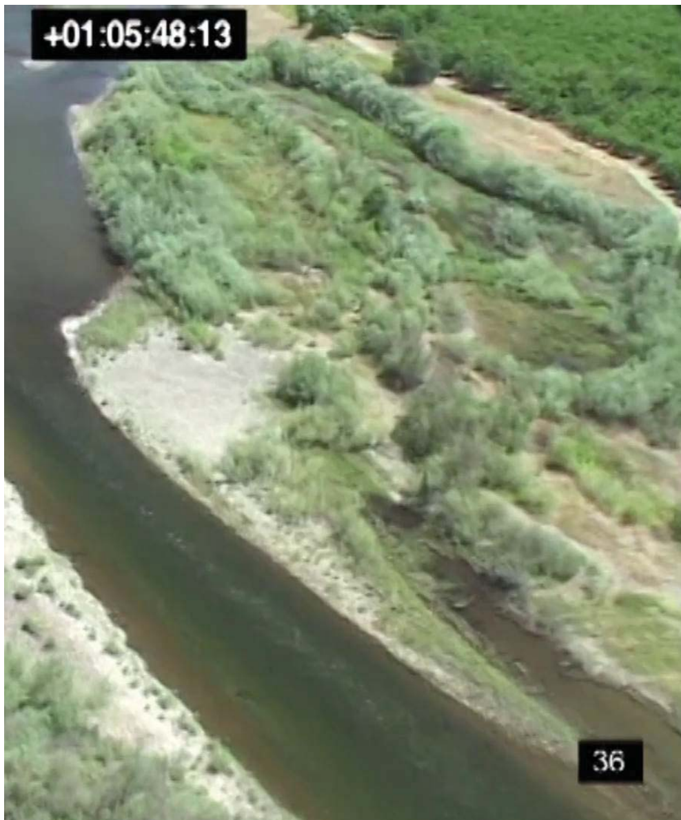
Figure 17. Mannings n is equal to .08.
