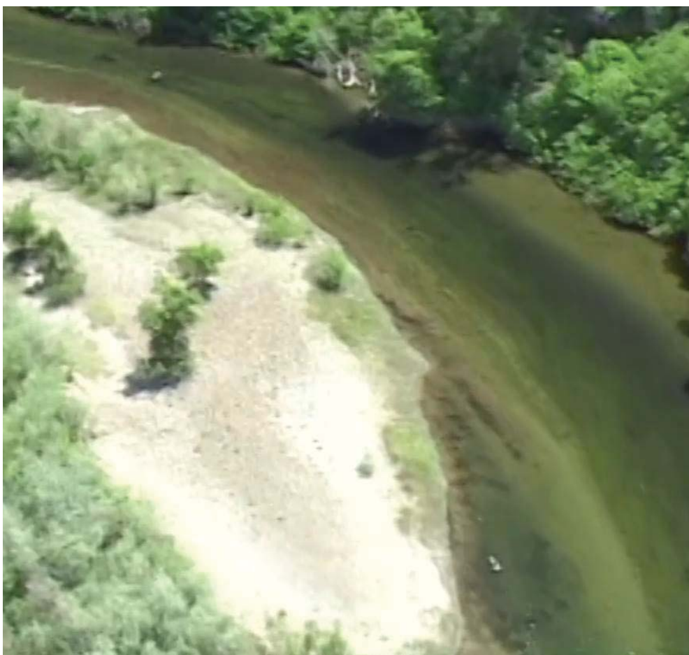
Figure 5. Mannings n is equal to .04.
