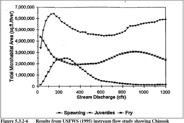
Figure 5.3.2-6Results from USFWS (1995) instream flow study showing Chinook<br/>salmon habitat in the lower Tuolumne River as a function of stream flow.Source: USFWS 1995.
