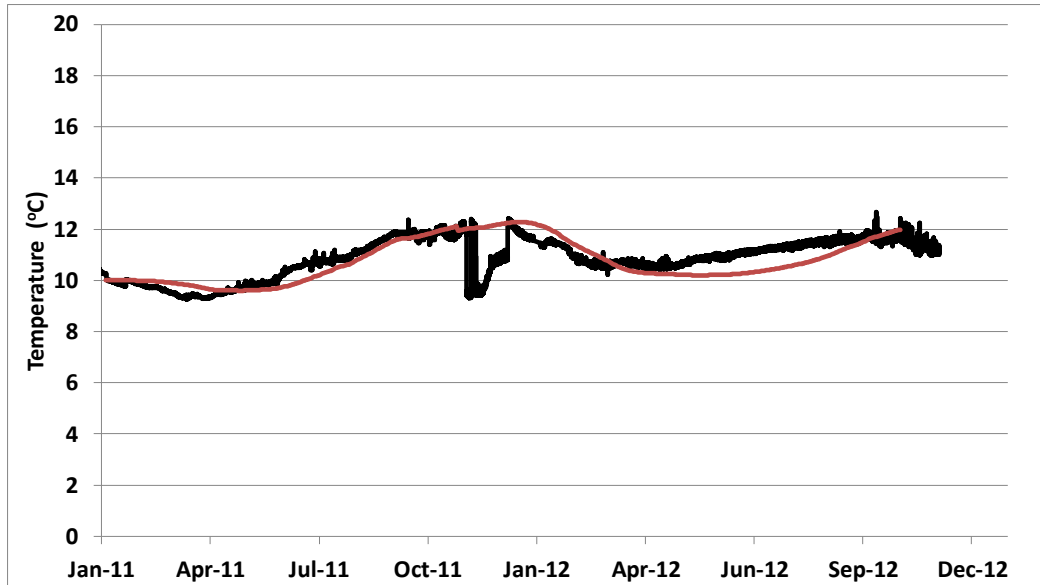
Figure 5.4-1. Measured and modeled outflow temperatures, 2011-12. (Measured = black; Modeled = red)
