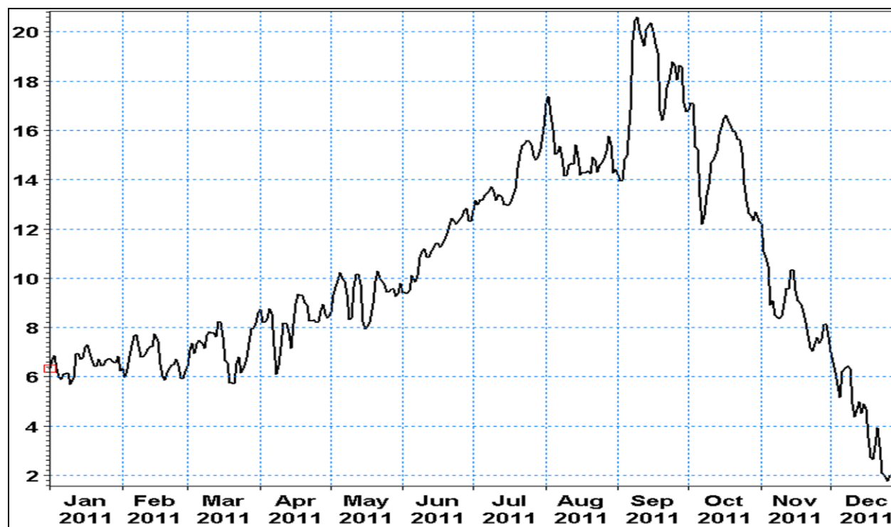
Figure 4.4-48. Measured inflow temperature at Indian Creek Trail (°C) for 2011.
