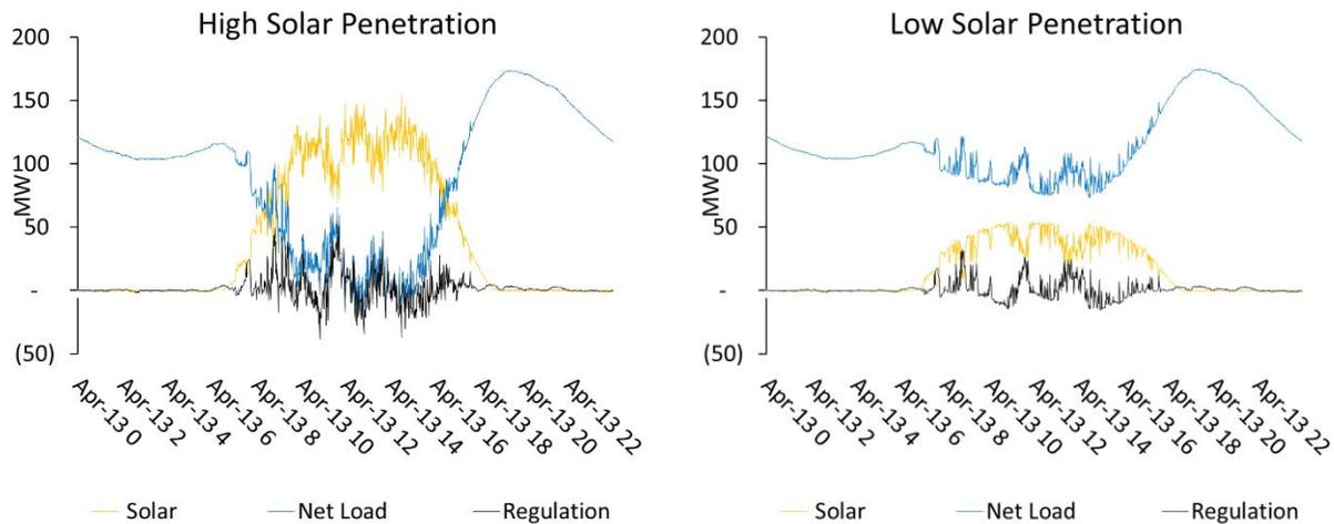
Figure 14: Comparison of regulation requirements for an energy system with higher and lower solar penetration.
