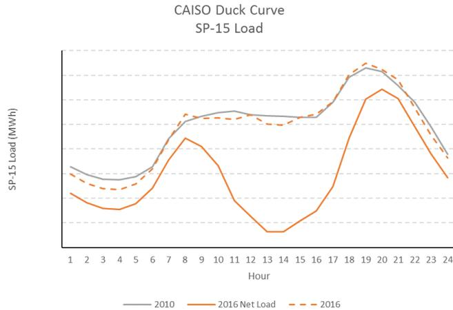
Figure 3: The Duck Curve - Solar generation's impact on load
