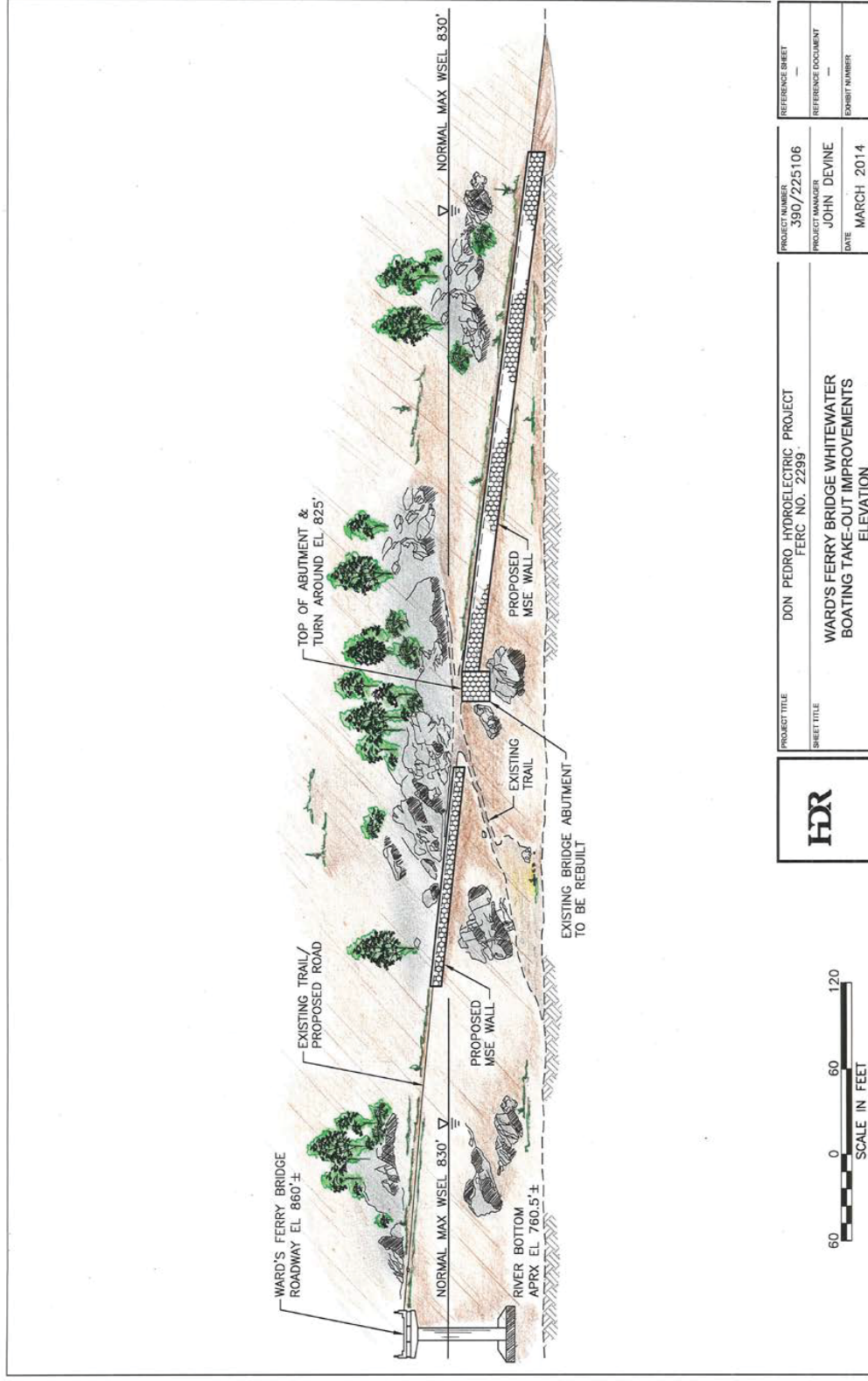
Figure 3.2-4. Ward's Ferry bridge whitewater boating take-out improvements – elevation view.
