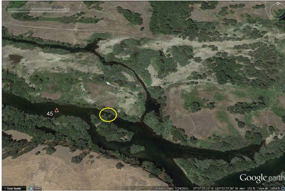
Figure 2. Artificial dam at RM 45.5. Dam seems to have been overtopped during preceding high flows but still can be seen through the water (2011 imagery, flow of 1,020 cfs) (Google 2013).
