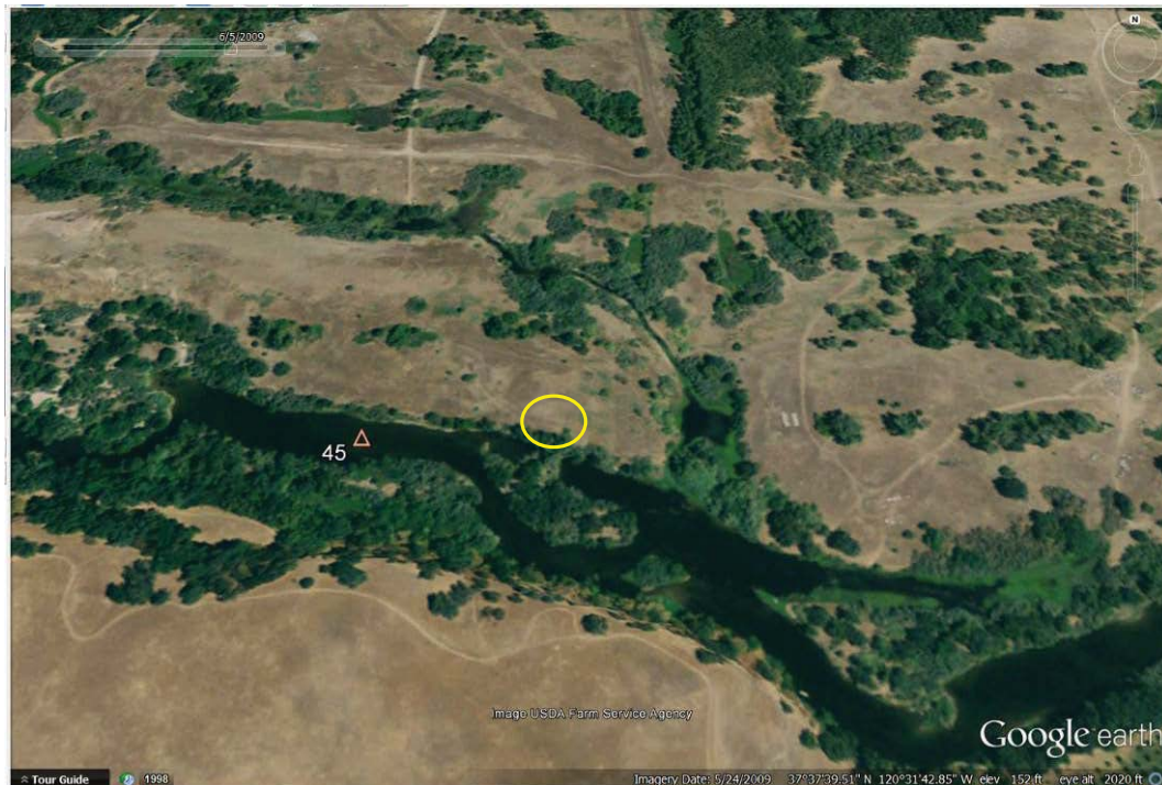
Figure 1. Artificial dam RM 45.5. Dam seems to be at floodplain stage or higher (2009 imagery, flow of 490 cfs) (Google 2013).
