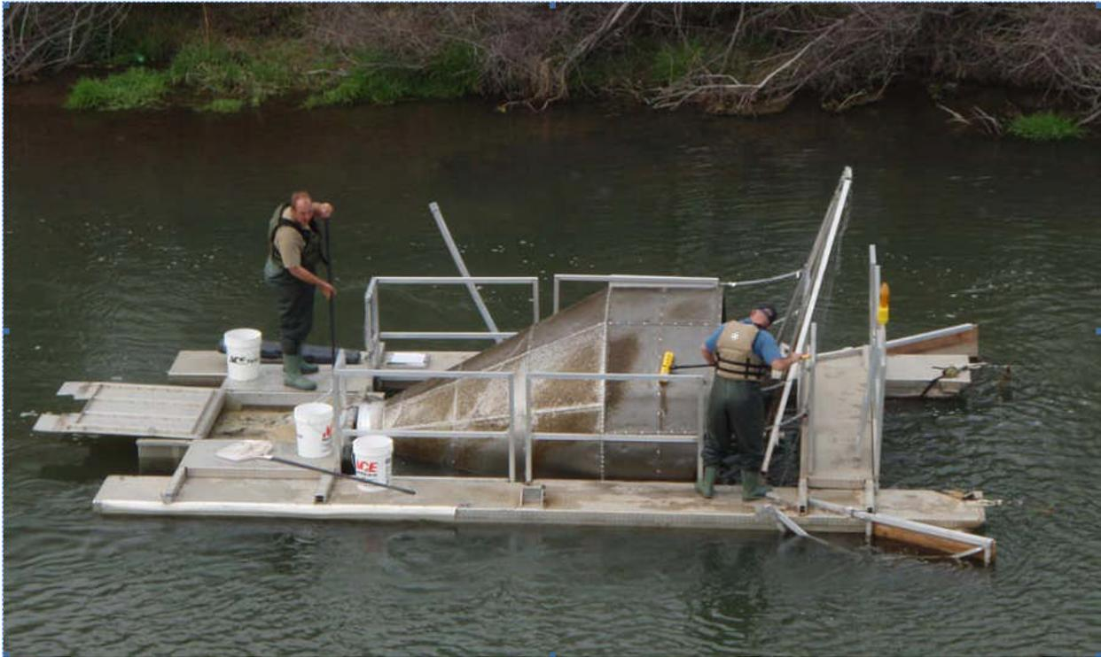
**Figure 5.3.2-5 Rotary screw trap in the lower Tuolumne River.**
